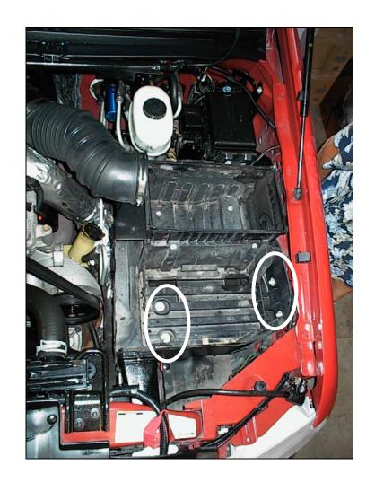
7) REMOVE THE FOUR BOLTS INSIDE THE BATTERY BOX...
