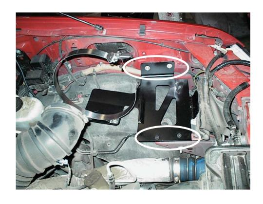
9) INSTALL THE UMP BATTERY TRAY IN THE STOCK LOCATION USING THE FORD BOLTS IN THE FENDER HOLES AND THE SUPPLIED COUNTERSUNK ALLEN BOLTS IN THE BATTERY TRAY.
