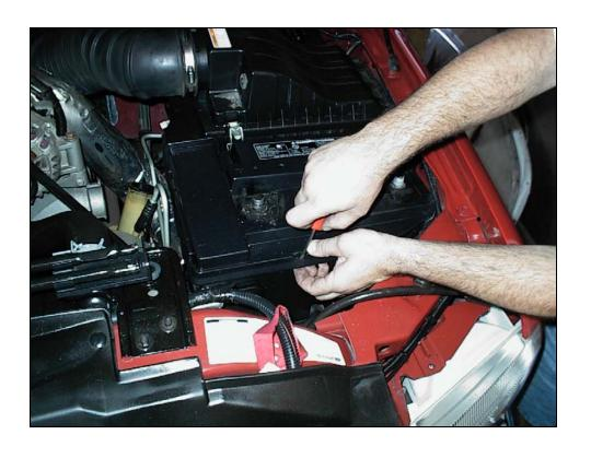
3) UNSNAP BATTERY COVER FROM DRIVERS' SIDE. THIS IS A REAL PAIN, STICKING A SCREWDRIVER IN THE SLOT HELPS.
