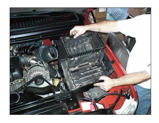
...AND LIFT OUT THE ENTIRE PLASTIC BATTERY/AIR BOX ASSEMBLY.
