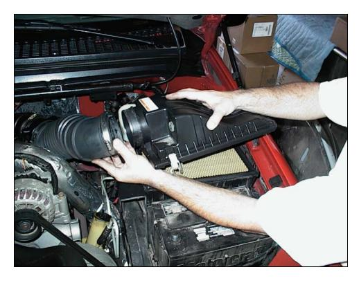
6) DISCONNECT THE AIR INTAKE HOSE FROM THE AIR BOX AND REMOVE AIR FILTER LID. PULL OUT THE FILTER GAUGE AND SAVE TO BE REUSED.
