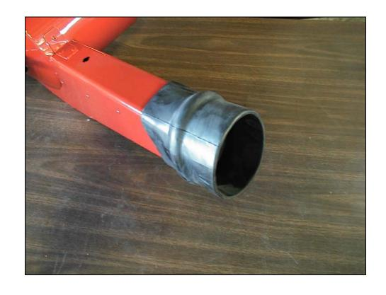
11) SLIDE THE PROVIDED RUBBER BELLOWS OVER THE INTAKE SNORKEL ABOUT HALFWAY. THIS WILL SEAL THE AIR INTAKE TO THE CORE SUPPORT AFTER INSTALLATION.
