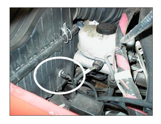
5) DISCONNECT THE INTAKE AIR TEMP SENSOR FROM THE REAR OF THE STOCK AIR BOX LOCATED ON THE BACK OF THE AIRBOX BY THE BRAKE MASTER CYLINDER, REMOVE THE SENSOR AND SAVE, THIS WILL BE REUSED IN THE UMP SUPERFILTER.
