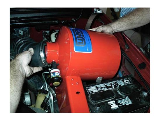
BEFORE THE FILTER CANISTER IS SEATED INTO THE CLAMP, START THE INTAKE HOSE ON TO THE NEW FILTER. IT IS A LITTLE TRICKY HOLDING THE FILTER UP SLIGHTLY AND GETTING THE HOSE STARTED.
