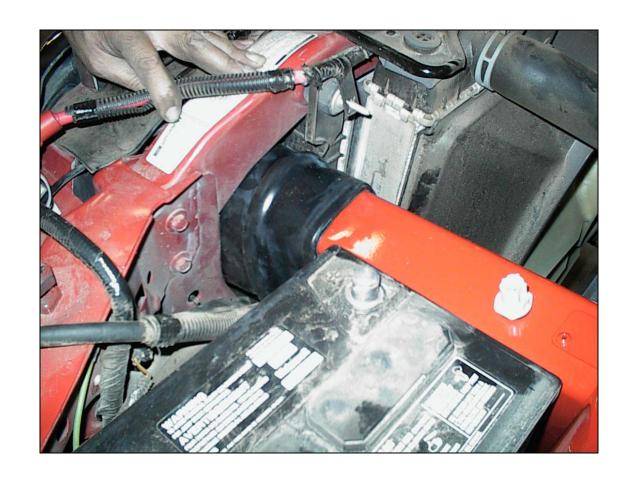
13) INSTALL THE FILTER ASSEMBLY CAREFULLY FEEDING THE RUBBER BELLOWS THROUGH THE STOCK HOLE NEXT TO THE RADIATOR. LIFT UP THE RUBBER FLAP IN FRONT OF THE CORE SUPPORT TO INSURE THE BELLOWS IS NOT PINCHED OFF OR FOLDED OVER.
