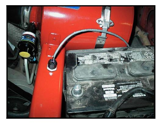
14) SAFELY ROUTE THE EXTENSION LOOM FOR THE INTAKE AIR TEMP SENSOR AND PLUG ON TO THE SENSOR. FAILURE TO DO THIS CAN CAUSE THE "CHECK ENGINE" LIGHT TO COME ON. IF YOU FORGET THIS AND THE LIGHT COMES ON, DON'T WORRY. DRIVING THE TRUCK FOR A WHILE AFTER PLUGGING IN THE SENSOR WILL CLEAR THE LIGHT.
