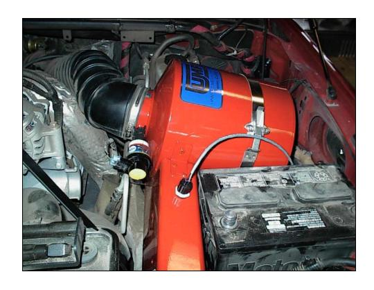
THE INTAKE HOSE WILL BE HARD AGAINST THE INTER COOLER PIPE AND WHILE THIS IS NOT THE BEST, IT HAS BEEN SHOWN TO BE NO PROBLEM IN TESTING. IF YOU ANTICIPATE FREQUENT FILTER MAINTENANCE, PUT SOME ANTI- SEIZE ON THE STOCK FORD HOSE CLAMP THREADS TO PREVENT GALLING OF THE STAINLESS STEEL CLAMP.
